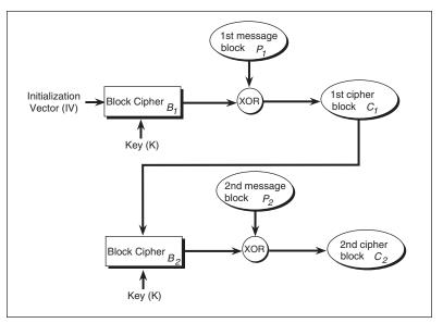
Figure 3-5 Cipher Feedback (CFB) Mode
