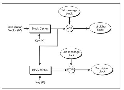
Figure 3-6 Output Feedback Mode (OFB)
