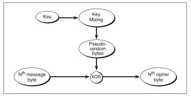
Figure 3-7 RC4 Encryption or Decryption
