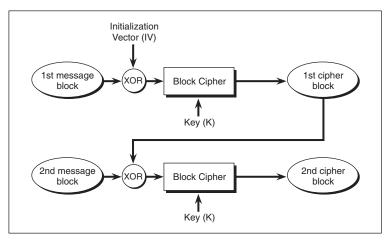
Figure 3-4 Cipher-Block Chaining (CBC) Mode
