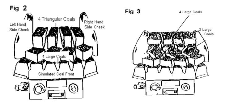
Lay 3 large coals in the gaps between the triangular coals and the row of 4 coals and place 4 large coals on the triangular coals behind the second row of coals as shown in Fig. 3 & 4.
