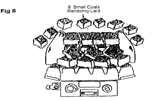
To obtain the best visual appearance it may be necessary to make slight adjustments to the position of the coals. NOTE: ADDITIONAL COALS MUST NOT BE USED
