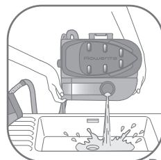
Rinsing out the boiler D
