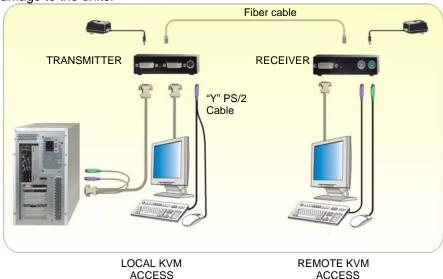
Figure 1. Typical cabling configurations
