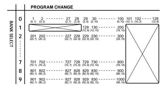
The program number indicated by the Bank and Number pedal values shown in parentheses is calculated in exactly the same way as for the Program Change numbers described in "About Program Change Numbers" (p. 11). That is, the Program number is the Bank multiplied by ten, plus the Number (Bank x 10 + Number).
