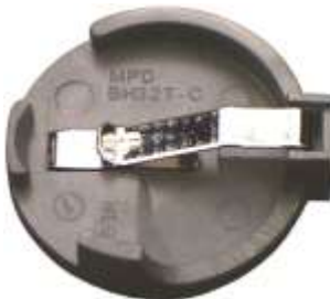
Battery Holder 20mm dia. coin cell
