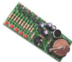
Pocket VU Meter (wireless) 3V
