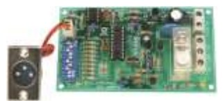
DMX-Controlled Relay Switch AD854 ... R 463.11
