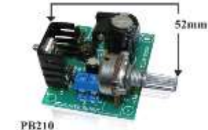
1.3 to 30V Adjustable Power Supply
