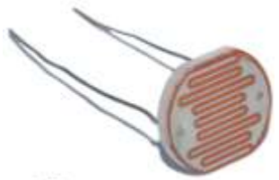
LDR Photoresistor 50-100kOhm 11mm Dia.
