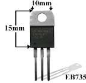
LM2940T-5 Reg low dropout +5V 1A (TO220)
