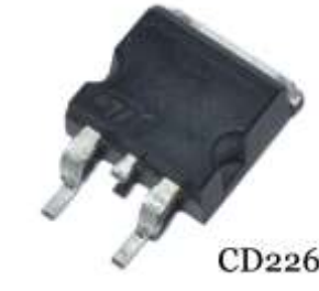
LM317D2T Regulator 1.2 to 37V 1.5A DPAK
