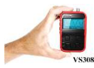
HPS140I Handheld Pocket Scope 40MS/sec VS308 a R 1404.2
