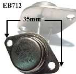
LM317K Regulator 1.2 to 37V 1.5A (TO3)
