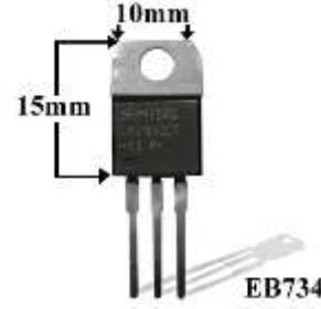
LM2940T-12 low dropout 12V 1A Reg. TO220
