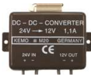
Voltage Converter 24V-12V 1.1A Module
