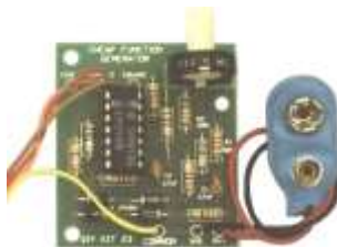
Op-Amp Function Generator 9VDC
