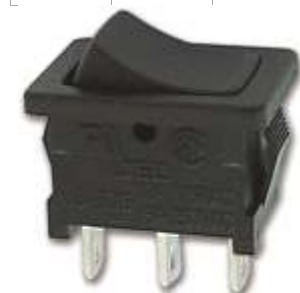
Rocker Switch 3A 250V 1P2T 13x19mm
