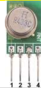
Transmitter Module TX433N AB341 P0527 R 163.26
