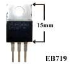
LM338T Regulator 1.3 to 32V 5A (TO220)
