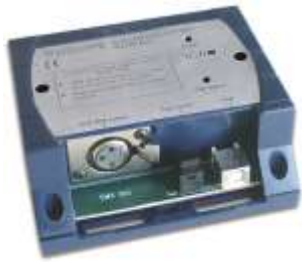
USB-Controlled DMX Interface Solder Kit
