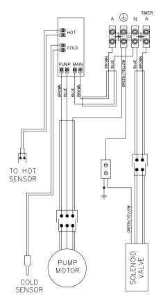
A double pole isolating switch must be incorporated in the fixed wiring, according to the AS/NZS 3000, AS 5601 and local authority requirements.
