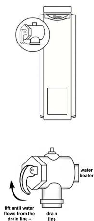
The temperature pressure relief valve should be checked for performance or replaced at intervals not exceeding 5 years, or more frequently in areas where there is a high incidence of water deposits (refer to "Water Supplies" on page 56).
