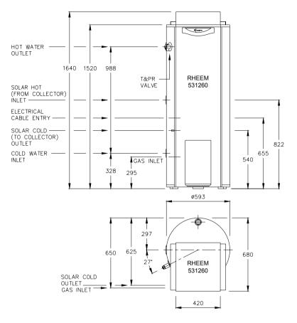
Model531260Mass (tank):Empty 110 kgFull 370 kgCapacity & Boost:260 litresRecovery (Boost)<br/>(natural gas @ 50°C rise)100 litres
