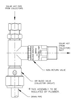
• Close the bleed valve when water runs freely from the drain line.
