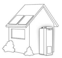
The installation must comply with the requirements of AS/NZS 3500.4, AS/NZS 3000, AS 5601 and all local codes and regulatory authority requirements. In New Zealand, the installation must conform with NZS 5261 Code of Practice for Installation of Gas Burning Appliances and the New Zealand Building Code.
