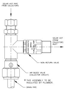
Close the bleed valve when water runs freely from the drain line.
