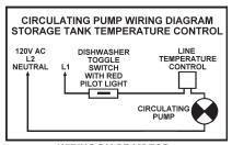
WIRING DIAGRAM FOR 180°F (82°C) LOOP (IF USED).
