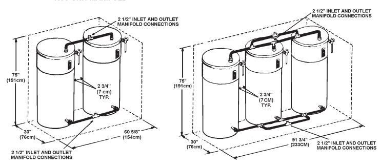
CAUTION: IF THE PLUMBING REQUIRES THE USE OF PIPES WITH DISSIMILAR MATERIAL (FOR EXAMPLE, STEEL AND COPPER), USE DIELECTRIC UNIONS TO PREVENTAN ELECTRO-GALVANIC ACTION BETWEEN THE PIPING COMPONENTS WITH DISSIMILAR MATERIALS.
