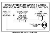
WIRING DIAGRAM FOR 180°F (82°C) LOOP (IF USED).
