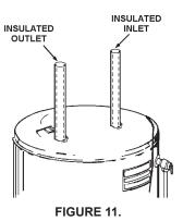
Fit pipe insulation over the incoming cold water line and the hot water line. Make sure that the insulation is against the top cover of the heater. Fit T & P valve insulation over valve. Make sure that the insulation does not interfere with the lever of the T & P valve.
