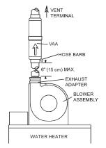
FIGURE 22: Typical Vertical Installation
