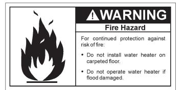
This water heater must not be installed directly on carpeting. Carpeting must be protected by metal or wood panel beneath the appliance extending beyond the full width and depth of the appliance by at least 3" (7.6 cm) in any direction, or if the appliance is installed in an alcove or closet, the entire floor must be covered by the panel. Failure to heed this warning may result in a fire hazard.
