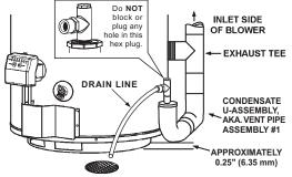
\*NO PORTION OF THE FIELD SUPPLIED DRAIN LINE BEYOND THE 1/2" ADAPTOR MAY BE ELEVATED HIGHER THAN THE ADAPTOR. THIS MUST BE TRUE FOR THE ENTIRE LENGTH OF DRAIN LINE INCLUDING EXIT INTO AN APPROPRIATE DRAIN.
