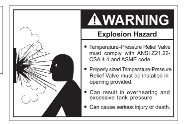
This water heater is provided with a properly rated/sized and certified combination Temperature-Pressure Relief Valve (T&P valve) by the manufacturer. The valve is certified by a nationally recognized testing laboratory that maintains periodic inspection of production of listed equipment of materials as meeting the requirements for Relief Valves for Hot Water Supply Systems, ANSI Z21.22 • CSA 4.4, and the code requirements of ASME.
