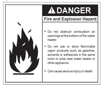
INSTALLED IN SUITABLE AREA: To insure sufficient ventilation and combustion air supply, proper clearances from the water heater must be maintained. See "Locating the New Water Heater" section. Combustible materials such as clothing, cleaning materials, or flammable liquids, etc. must not be placed against or adjacent to the water heater which can cause a fire.
