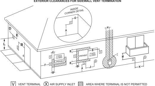
**POWER VENT** (using room air for combustion) EXTERIOR CLEARANCES FOR SIDEWALL VENT TERMINATION
