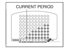
The speed setting for the first period is shown in the flashing CURRENT PERIOD column of the LED matrix. (The incline settings are not shown in the matrix.)
