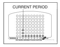
ting for the first period is shown in the flashing CURRENT PERIOD column of the LED matrix. (The incline settings are not shown in the matrix.) To program speed and incline settings for the first period, simply adjust the speed and incline of the treadmill to the desired levels with the SPEED and INCLINE buttons. Every few times a SPEED button is pressed, an additional indicator will light or darken in the CURRENT PERIOD column.
