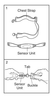
Next, wrap the heart rate monitor around your chest and attach the other end of the chest strap to the sensor unit.
