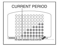
speed and/or incline setting may be programmed for consecutive periods.) The speed setting for the first period is shown in the flashing CURRENT PERIOD column of the LED matrix. (The incline settings are not shown in the matrix.) The speed settings for the next seven periods are shown in the seven columns to the right.
