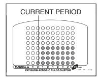
setting for the first period will be shown in the flashing CURRENT PERIOD column of the LED matrix. The target heart rate settings for the next seven periods will be shown in the seven columns to the right.
