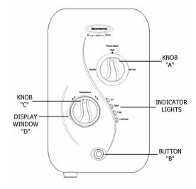
During normal operation, if an overheated water temperature is sensed then the heater will switch off and the "Overheat" light will illuminate.
