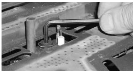
Remove the 2 screws, push Burner Tray to the left, and lift off.
