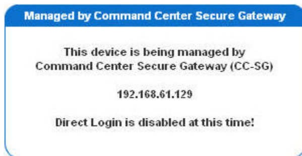
Figure 104: Device Managed by CC-SG Message
