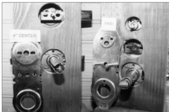
9. The photograph above illustrates the differences between the H and J series door preps and mounting plates.
