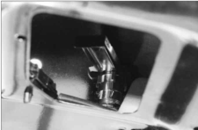
12. A horseshoe clip holds the trunk lock in place.
