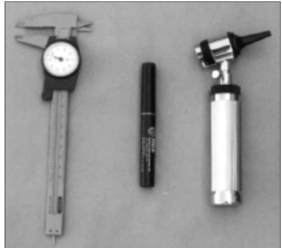
3. Other tools that are useful and can be carried in another box include a caliper, otoscope, moto tool, and a pen light.
