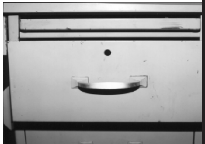
2. Drill a pilot hole and enlarge it to 1/2".
