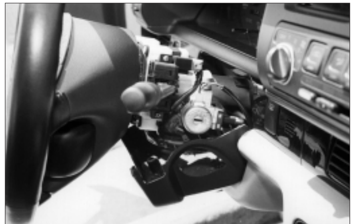
3. Removing the two piece clam shell shroud exposes the lock.
