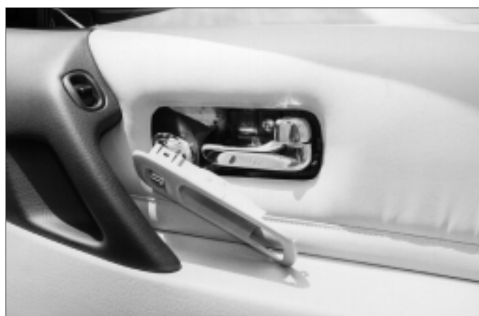
9. Unsnap and remove the handle.
