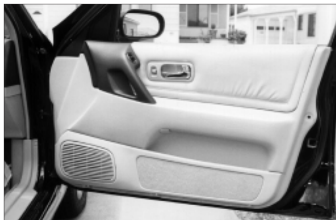
7. Make sure and remove all of the fasteners before removing this door panel.
