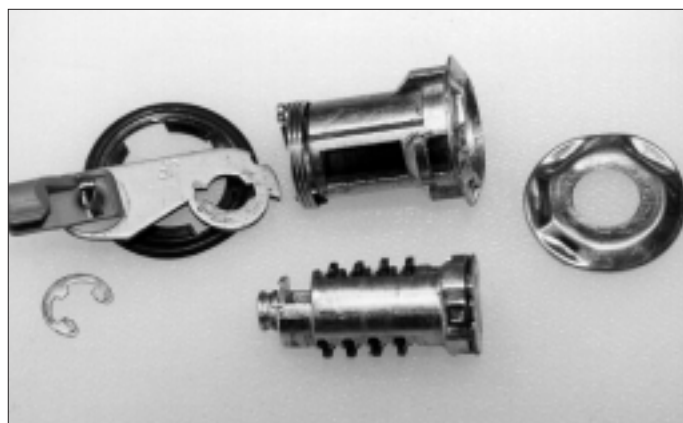
11. The door lock disassembled. If necessary, the tumblers can be read through the drain hole on the bottom of the cylinder.
