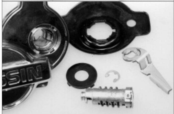
13. Remove the rubber gasket from the lock. Then use a small screw driver to unsnap the face cap tabs. The lock can now be disassembled.
