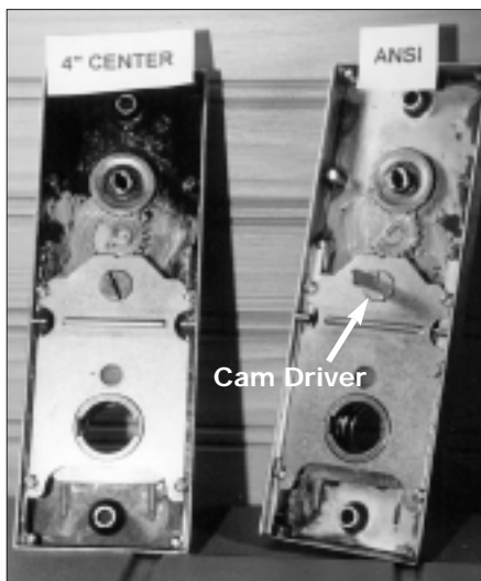
2. Inside the escutcheon of the J and K (ANSI) series. Notice the cam driver on the K series.
