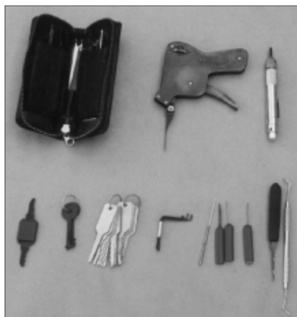
2. Tools are a locksmith's identity. Here are various tools that I keep in box. Included are various picks, broken key pullers, and try out keys.
