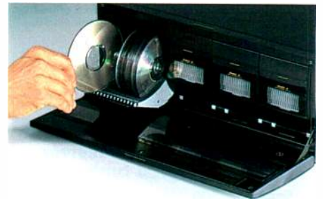
The CD-100's front panel swings down to reveal four vertical disc racks, each of which rolls out to hold up to 25 CDs. You can insert or remove discs in three racks at once (up to 75 CDs, total) without interrupting play of discs in the fourth.
