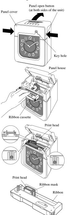
1 Unlock the unit. While holding down the panel, open buttons at both sides of the unit, and lift the panel cover away from you.
