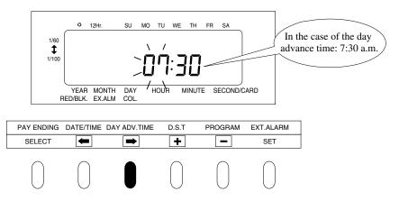
3 Check the settings on the display and press SET. Now the setting is completed.
