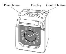
3 Make settings using the display and control buttons at the panel house.
