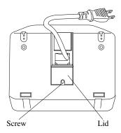
1 Unscrew the screw fixed on the bottom of the unit to remove the lid
