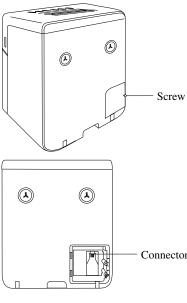
1 Unscrew the screw that holds the lid of the battery compartment in the lower right-hand corner of the back of the unit.
