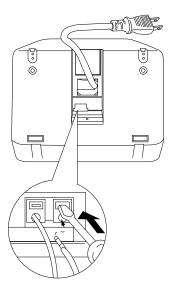
2 Insert two wires for an external time signal while pushing the upper part of the terminal board with a screwdriver.
