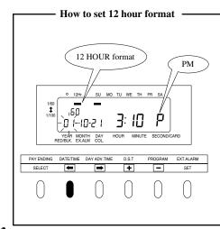
When you want to apply 12 hour format both on LCD time and printing format on the time card, select 12 hour format first as described below.
