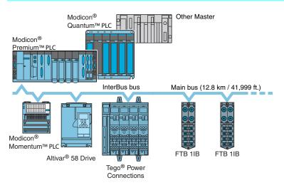
InterBus is a serial link type fieldbus for sensors and actuators which satisfies the requirements of industrial environments.
