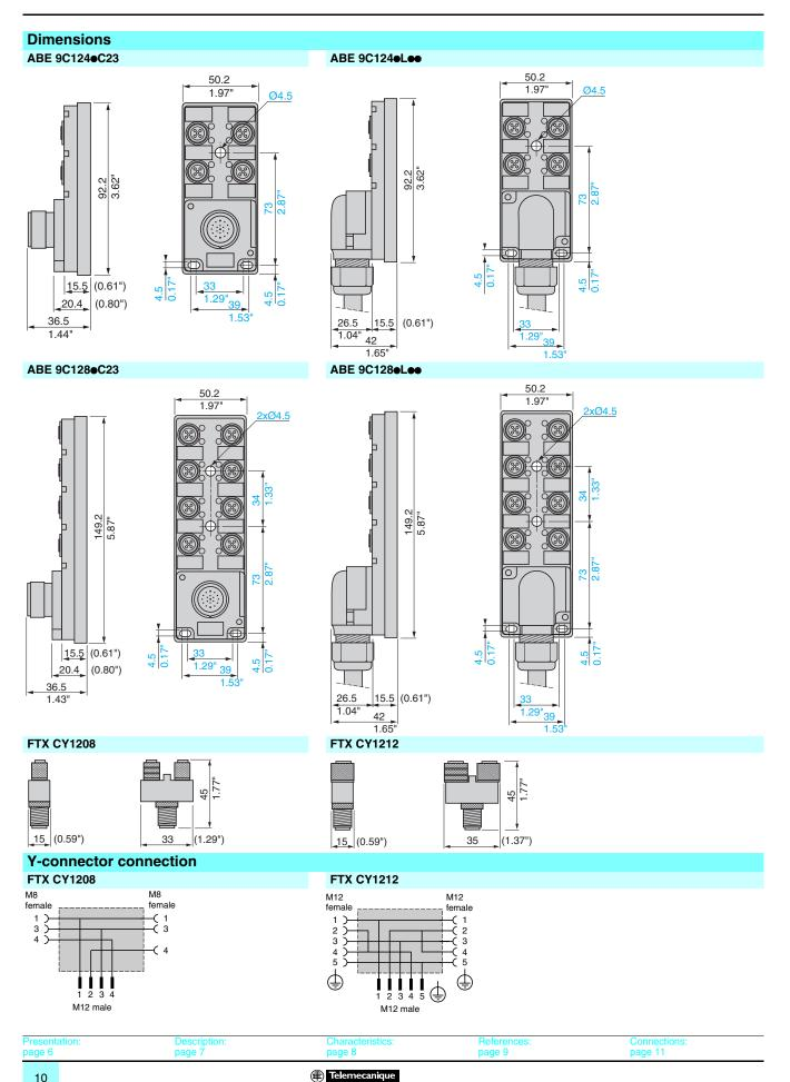
**IP 67 passive splitter boxes** Telefast<sup>®</sup> Distribution System, ABE9 splitter boxes
