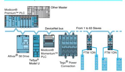
The DeviceNet system is a sensor/actuator bus system of the open Low-End type, used in various industrial applications and, in particular, the automobile industry. It is based on CAN technology (OSI layers 1 and 2).
