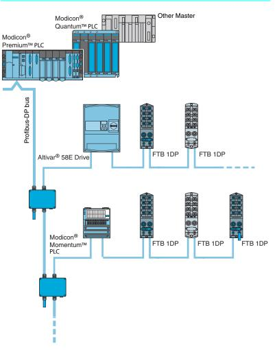
The Profibus-DP (Process Fieldbus Decentralized Peripheral) is an open type fieldbus system for industrial applications. The Profibus standard is described in standard EN 50170.
