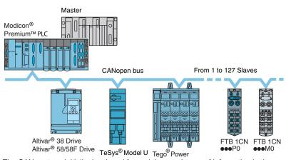
The CAN system, initially developed for real-time exchange of information in the automobile industry, is now being used more and more throughout industry. There are several fieldbuses based on CAN base layers and components.
