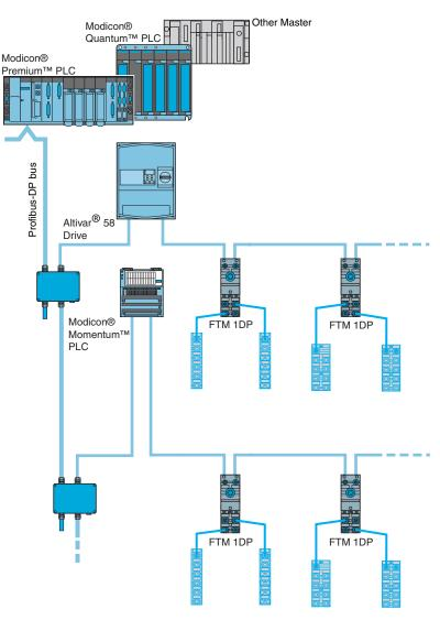
The Profibus-DP (Process Fieldbus Decentralized Peripheral) is an open type fieldbus system for industrial applications. The Profibus standard is described in standard EN 50170.
