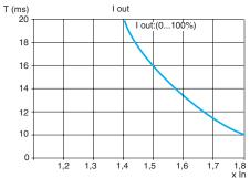
Example: For an ABL 7UPS24eee power supply with 50 % loading. (I out = 50 %), this power supply can absorb a current peak of 1.6 x In for 250 ms with an output voltage  $\geq$  19 V.
