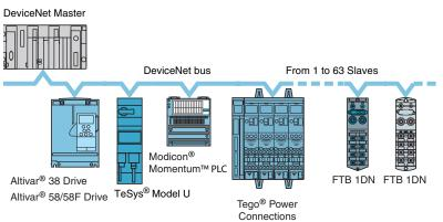
The DeviceNet system is a sensor/actuator bus system of the open Low-End type, used in various industrial applications and, in particular, the automobile industry. It is based on CAN technology (OSI layers 1 and 2).
