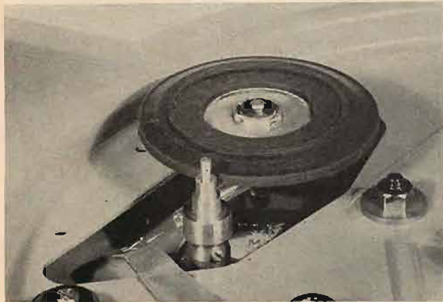
The drive system should be as simple as possible. This one has only a stepped motor pulley and a rubber-rimmed idler.
