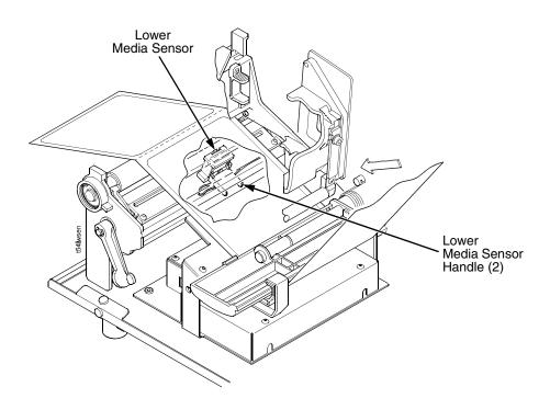
Your printer is equipped with upper and lower media sensors that detect the top-of-form position on media with label length indicators (gaps, notches, holes, or black marks). The media sensors also detect Paper Out conditions.
