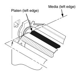
12. Align the left (inside) edge of the media with the left straight edge of the platen (rubber drive roller).
