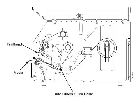
4. Thread the end of the ribbon under the rear ribbon guide roller, then between the platen and the printhead.
