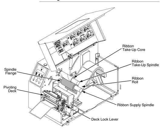
1. Install the ribbon take-up core on the ribbon take-up spindle.
