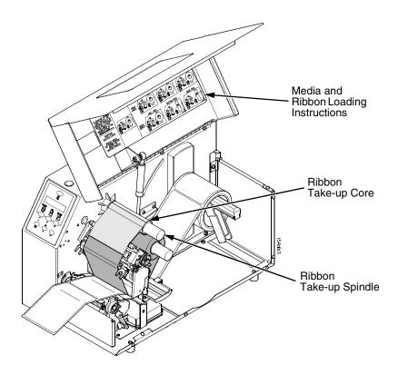
5. Route the ribbon as illustrated on the media and ribbon loading instructions (or refer to the arrows on the printer frame).
