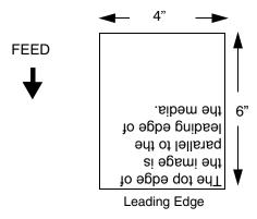
• Inv. Portrait. Inverse Portrait refers to vertical page orientation, where the height of a page is greater than its width. The top edge of the image is parallel to the trailing edge of the media. The following example is viewed from the front of the printer.
