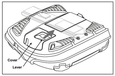
Figure 13 - Removing The Universal Port Cover
