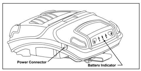
Figure 10 - Power Connector & Battery Indicator
