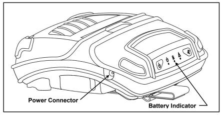
Figure 3 - Power Connector & Battery Indicator
