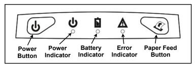
**Figure 5 - Printer Control Panel**
