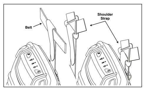
Figure 7 - Carrying Strap on Belt or Shoulder Strap
