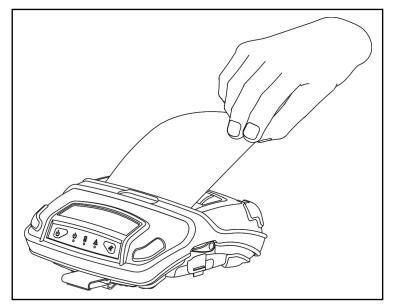
Figure 6 - Tearing Off Printer Output
