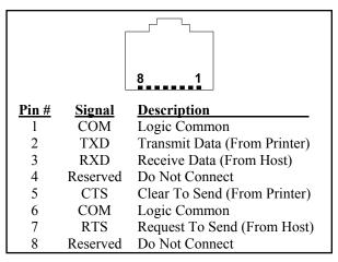
Figure 15 - Connector Pin Assignments
