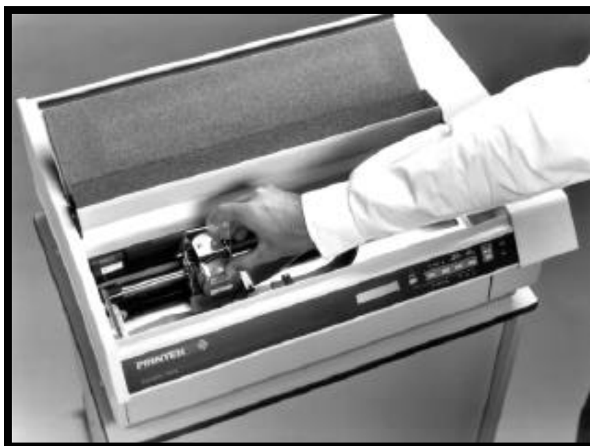
Lowering (closing) Ribbon Loading Bail.
