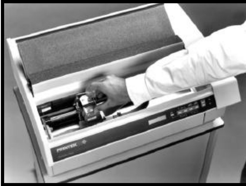
Lowering (closing) Ribbon Loading Bail.
