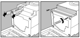
Set the machine upright and remove the two remaining bolts from the back.
