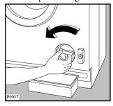
Unscrew and remove the filter. Clean carefully under a fast running tap.
