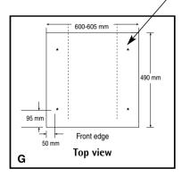
Position the base into the recess with its front edge as far forward as the adjoining plinth line will allow. The reason for placing the base in this position is to allow a small strip of beading to be fitted in front of the appliance feet. Fix the base firmly to the floor using four appropriate countersunk screws (see Fig. H).
