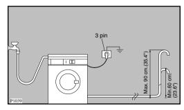
Make sure that it is designed in such a way, that the end of the drain hose cannot be covered with water. The drain hose may be extended to a maximum of 4 metres. An additional drain hose and joining piece is available from your local Service Force Centre. The joining piece must have an internal diameter of 18mm. If you intend the drain hose to empty into a sink, make sure that the sink is empty and the plug hole is not blocked. Use the plastic "U-Piece" supplied.
