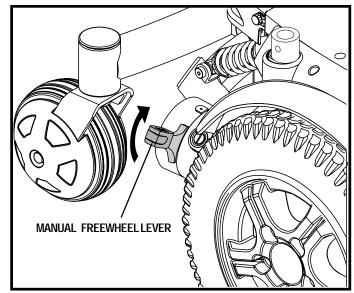
Figure 9. Drive Mode (Drive Engaged)
