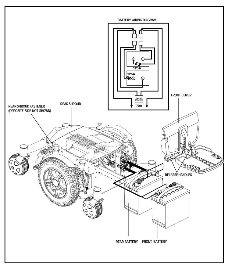
Figure 29. Battery Installation
