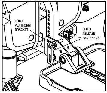
Figure 20. Foot Platform Adjustment
