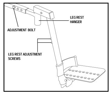
Figure 25. Heavy Duty Drop-In Leg Rests
