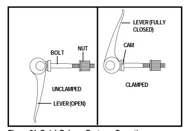
Figure 21. Quick Release Fastener Operation
