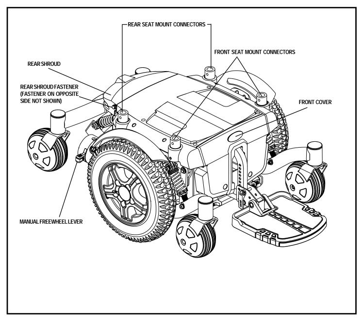
Figure 6. The Quantum 6000Z Series Power Base
