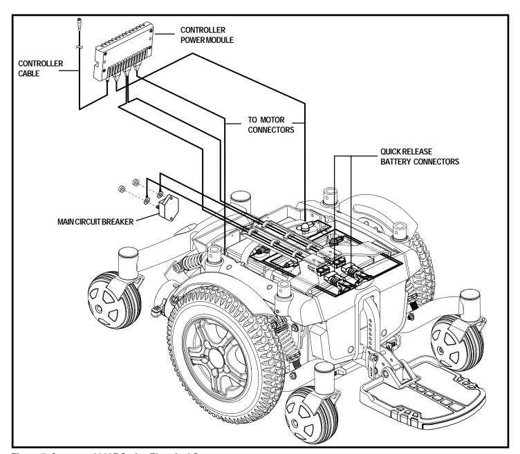
Figure 7. Quantum 6000Z Series Electrical Components
