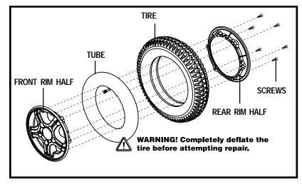
Figure 27. Quantum 6000Z Series Drive Wheel
