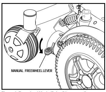
Figure 8. Freewheel Mode (Drive Disengaged)
