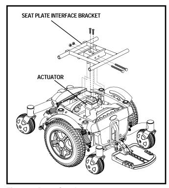
Figure 14. Power Seat Actuator
