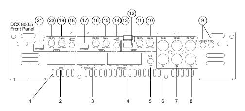
**1. Cooling Plenums:** Maintain a minimum 2" clearance around cooling plenums for proper amplifier cooling.
