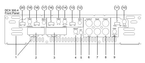
**1. Cooling Plenums:** Maintain a minimum 2" clearance around cooling plenums for proper amplifier cooling.
