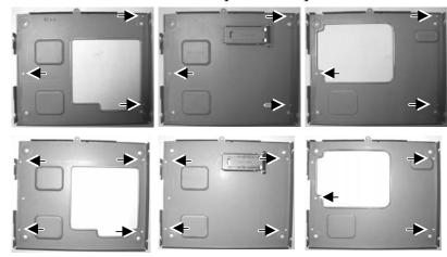
mechanical fixation parts in the wall mount bracket and hang the backpack to the back cover that is already fixed on wall with the cables coming out of the brackets through the openings marked with rectangles in the top row pictures above. Screw lock the top side of the backpack.
