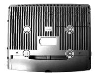
slide down the winding grooves in the wall mount backpack. Connect all cables coming out of the backpack into the cable cover area of main unit.
