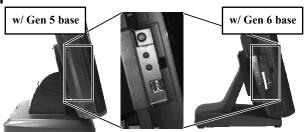
the + or – button changes the LCD panel display brightness by a small amount. When you press and hold the button the change will keep on until release or extreme condition matched. It is preferable to keep this cover closed in daily operation. The LCD brightness can also be controlled through software setting.
