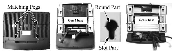
Match the matching pegs on the back of the main unit against the (rectangular marked above for both base types) matching holes on the stand assembly. First aim the matching pegs toward the upper round part of the hole (ref. the close-up illustration) and make sure that all pegs are inside the holes.
