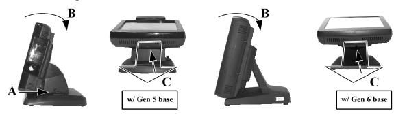
**Step A:** Push lock/release lever of the Gen 5 slim base for tilt angle adjust backward. (This operation is not required in Gen 6 super slim base)
