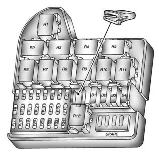
Instrument Panel Fuse Block - Fuse Puller Shown
