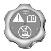
2. Locate the radiator pressure cap (B).
