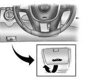
Pull the release handle with the above symbol on it. It is located below the instrument panel to the left of the steering wheel.
