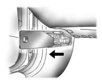
The instrument panel fuse block is located on the end of the instrument panel, on the driver's side of the vehicle. To access the fuses, open the fuse panel door by pulling out.
