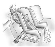
5. To tighten the belt, push down on the child restraint, pull the shoulder portion of the belt to tighten the lap portion of the belt, and feed the shoulder belt back into the retractor. If you are using a forward-facing child restraint, you may find it helpful to use your knee to push down on the child restraint as you tighten the belt.
