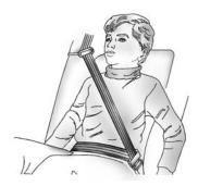
4. Buckle, position, and release the safety belt as described previously in this section. Make sure that the shoulder belt crosses the shoulder.
