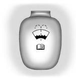
Open the cap with the washer symbol on it. Add washer fluid until the tank is full. See *Engine Compartment Overview on page 9-6* for reservoir location. Notice:
