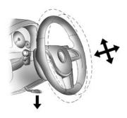
The adjustment lever is located on the left side of the steering column.
