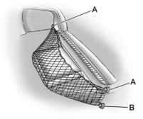
To create a pouch, attach the four corner loops (A) to each of the two top hooks. Attach the nets center loops (B) to the bottom hooks.
