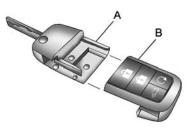
The key is purchased as two sections: the key blade and immobilizer section (A) and the remote keyless entry and remote start system section (B).
