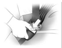
To unlatch the belt, push the button on the buckle. The belt should go back out of the way. When the safety belt is not in use, slide the latch plate up the safety belt webbing. The latch plate should rest on the stitching on the safety belt, near the guide loop on the side wall. Before you close a door, be sure the belt is out of the way. If you slam the door on it, you can damage both the belt and the vehicle.
