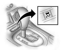
The ESP button is located in front of the transmission gear selector lever.
