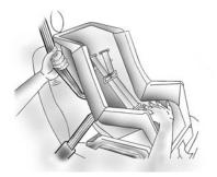
6. To tighten the belt, push down on the child restraint, pull the shoulder portion of the belt to tighten the lap portion of the belt and feed the shoulder belt back into the retractor. If you are using a forward-facing child restraint, you may find it helpful to use your knee to push down on the child restraint as you tighten the belt. 7. Push and pull the child restraint in different directions to be sure it is secure.
