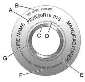
Passenger (P-Metric) Tire Example (A) Tire Size: The tire size is a combination of letters and numbers used to define a particular tire's width, height, aspect ratio, construction type, and service description. See the "Tire Size" illustration later in this section for more detail.
