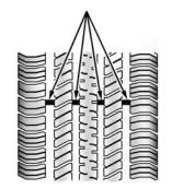
One way to tell when it is time for new tires is to check the treadwear indicators, which will appear when the tires have only 1/16 inch (1.6 mm) or less of tread remaining. You need new tires if any of the following statements are true:
