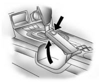
To set the parking brake, pull up on the parking brake handle. If the ignition is in the ON/RUN position, the brake system warning light will come on. See *Brake System Warning Light on page 4-16*. To release the parking brake:
