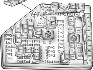
Engine Compartment Fuse Block - Fuse Puller Shown
