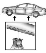
Position the jack lift head at the jack location nearest the flat tire. The location is indicated by a mark on the bottom edge of the vehicle. The jack must not be used in any other positions.
