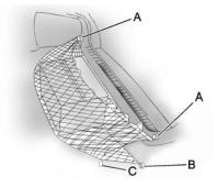
To install the net, attach each of the corner loops (A, B) to the four hooks inside the trunk, leaving the center loop (C) unhooked.
