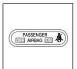
The passenger sensing system will turn off the right front passenger's frontal airbag and seat-mounted side impact airbag (if equipped) under certain conditions.
