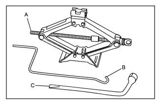
The tools you will be using include the jack (A), jack handle (B) and wheel wrench (C).
