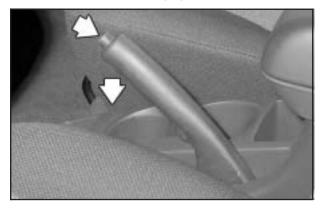
To release the parking brake, hold the brake pedal down. Pull the parking brake lever up until you can press the release button. Hold the release button in as you move the lever all the way down. *Notice:* Driving with the parking brake on can overheat the brake system and cause premature wear or damage to brake system parts. Verify that the parking brake is fully released and the brake warning light is off before driving.
