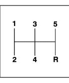
**FIRST (1):** Press the clutch pedal and shift into FIRST (1). Then, slowly let up on the clutch pedal as you press the accelerator pedal.
