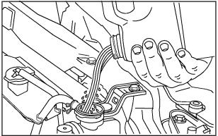
3. Fill the radiator with the proper coolant mixture, up to the base of the filler neck. See Engine Coolant on page 5-26 for more information about the proper coolant mixture.
