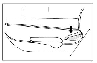
To adjust the seatback, lift the lever located on the outboard side of the seat. Release the lever to lock the seatback where you want it. Push on the seat to make sure it is locked into position. Pull up on the lever without pushing on the seatback, and the seat will go to its original upright position.
