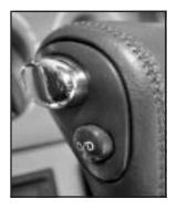
Your automatic transaxle has an O/D (overdrive off) button located on the left side of the shift lever.
