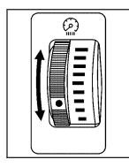
The instrument panel brightness control is located to the left of the steering wheel on the instrument panel. Turn the wheel on the left of the control up or down to increase or decrease brightness. Turn the wheel all the way up for the maximum setting. It is recommended that the brightness level be kept at the maximum setting for all daytime driving to ensure proper visibility.
