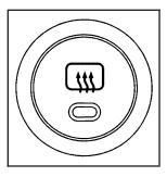
The rear window defogger button is located on the center of the instrument panel, above the audio system. The defogger does not operate with the rear liftglass opened.
