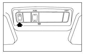
If the vehicle has a sunroof, it can be opened or put in a tilt position. To tilt the sunroof, slide the sunshade rearward, then press the switch marked UP. Press the other end of the switch to lower the sunroof. The ignition must be in the ON position for the switch to work.
