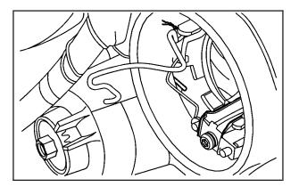
3. Release the retainer clip holding the bulb on the headlamp by pressing down and moving the metal retainer away from you.
