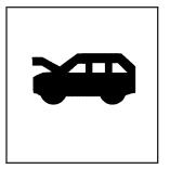
1. Pull the release handle with this symbol on it. It is located below the instrument panel to the left of the steering wheel.
