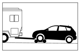
If your vehicle is a front-wheel drive vehicle it can be towed using a dolly. To tow your vehicle using a dolly, follow these steps:
