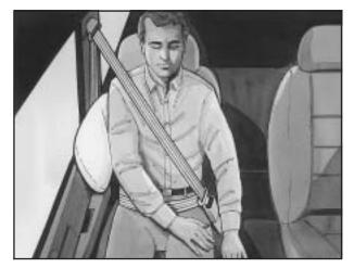
If your vehicle has a seat-mounted side impact airbag for the right front passenger, it is in the side of the passenger's seatback closest to the door.
