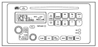
The radio has a blinking red light that is used as a theft-deterrent feature. The light will blink whenever the ignition is off.
