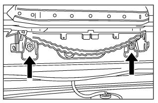
3. Remove the two screws from the CHMSL housing. Then remove the housing to expose the bulb.
