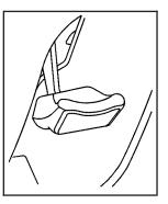
The tilt lever is located underneath, on the left side of the steering wheel column.
