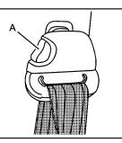
To move it down, squeeze the button (A) and move the height adjuster to the desired position. You can move the height adjuster up just by pushing up on the shoulder belt guide.
