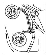
2. Turn the bulb socket counterclockwise and pull it out of the lamp housing.
