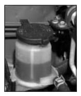
The power steering fluid reservoir is located in the engine compartment on the passenger's side of the vehicle. See *Engine Compartment Overview on page 5-12* for reservoir location.
