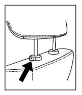
Press the release button at the base of the head restraint and push the restraint down to lower it.
