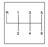
**FIRST (1):** Press the clutch pedal and shift into FIRST (1). Then, slowly let up on the clutch pedal as you press the accelerator pedal.
