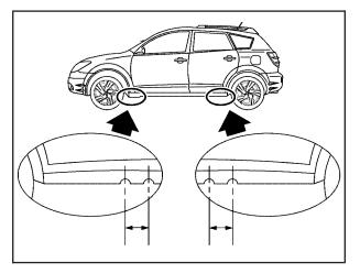
4. Position the jack and raise the jack lift head to fit over the car flange between the two notches.
