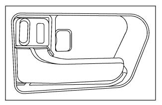
To manually lock the door from the inside, press the knob on the door forward. To unlock the door, press the knob rearward. With manual locks, you must use the key to lock and unlock the liftgate.
