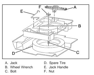
Return the jack (A), jack handle (E), wheel wrench (B) and compact spare tire to the storage area. When storing the compact spare tire, put it in place with the inner side of the wheel facing up.
