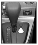
2. Carefully pry the cover from the shift lock override, located to the right of the shift lever.
