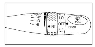
The lever on the right side of the steering column controls the windshield wipers and washer.
