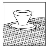
Pull up on the lock release knob, located on the top outboard side of the seatbacks.
