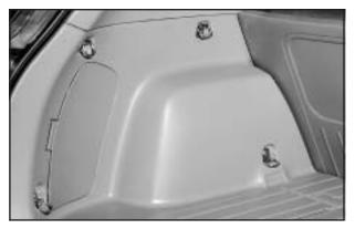
1. Remove the storage compartment cover in the rear cargo area of the vehicle to access the bulbs.
