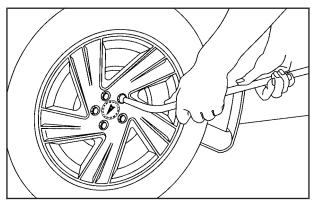
3. Using the wheel wrench, loosen all the wheel nuts. Do not remove them yet.
