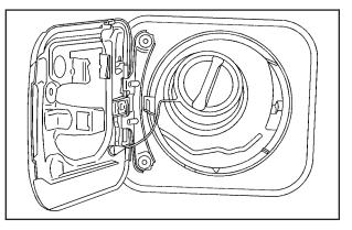
The tethered fuel cap is located behind a hinged fuel door on the driver's side of the vehicle.
