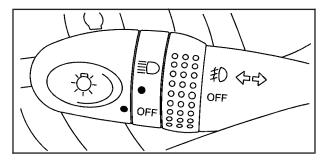
The turn signal/multifunction lever is located on the left side of the steering column.
