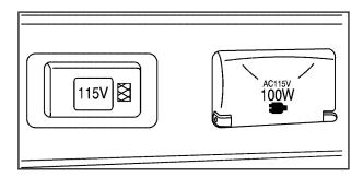
The power outlet is located near the center of the instrument panel. Before using the outlet, turn on the ignition and press the button next to the outlet. An indicator light in the button will come on. After using the outlet, press the button again to turn it off.
