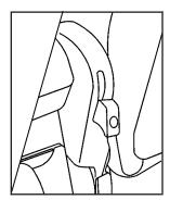
2. Pull up on one of the levers located on either side of the back of the passenger's seatback.
