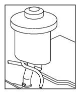
The hydraulic clutch and brake master cylinder use the same reservoir. It is filled with DOT-3 brake fluid. See *Engine Compartment Overview on page 5-12* for the location of the reservoir.
