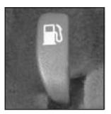
The fuel door release lever is located near the floor under the driver's seat on the outboard side. To remove the fuel cap, turn it slowly counterclockwise. On some vehicles you may have to push in while turning the cap.
