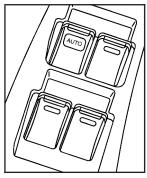
If your vehicle has this feature, the switches controlling the driver's and passenger's windows are located on the driver's door.
