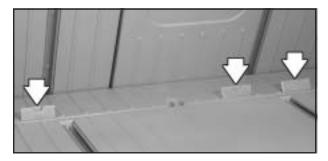
The top tether anchors are located on the floor of the rear cargo area. Flip open the trim cover to access the anchors. Be sure to use an anchor located on the same side of the vehicle as the seating position where the child restraint will be placed.
