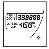
The button located on the right side of the instrument panel cluster allows you to switch between the odometer and the two trip odometers.
