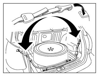
4. Hook the straps (end closest to the buckle) to the rear, upper tie-down hooks.
