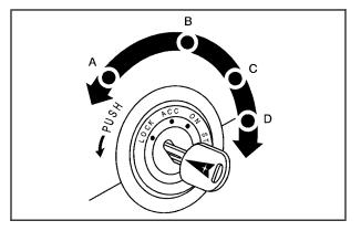
*Notice:* If your key seems stuck in LOCK and you cannot turn it, be sure you are using the correct key; if so, is it all the way in? If it is, then turn the steering wheel left and right while you turn the key hard. Turn the key only with your hand. Using a tool to force it could break the key or the ignition switch. If none of these work, then your vehicle needs service.
