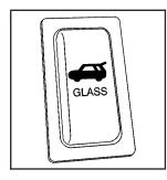
Your vehicle may have a liftglass release button which is located on the instrument panel to the left of the steering wheel. Press this button to release the liftglass.
