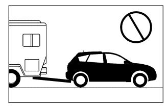
Do not tow your vehicle from the rear. Your vehicle could be badly damaged and the repairs would not be covered by your warranty.
