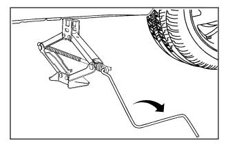
5. Raise the vehicle by turning the jack handle clockwise. Raise the vehicle far enough off the ground so there is enough room for the compact spare tire to fit underneath the wheel well.
