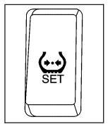
3. If the low-tire pressure warning light is on, push the SET (reset) button for a few seconds. The low-tire warning light should go off. The reset button is on the instrument panel to the left of the steering wheel. 4. Press and hold the SET (reset) button until the low-tire warning light comes on and flashes on/off three times. The tire pressure warning reset button starts the reset (initialization) process.
