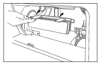
3. Lift the snaps on the filter cover to remove the cover.
