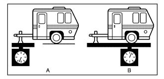
If you're using a weight-carrying hitch or a weight-distributing hitch, the trailer tongue (A) should weigh 10 to 15 percent of the total loaded trailer weight (B).
