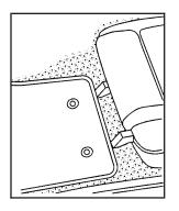
To remove the floor mat, pull up on the rear of the mat to disconnect it from the locator hooks.
