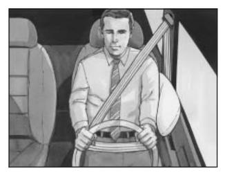
If your vehicle has a seat-mounted side impact airbag for the driver, it is in the side of the driver's seatback closest to the door.
