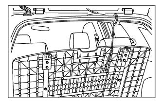
2. Lift up the cargo area floor panel, remove the hook attached to the bottom side of the panel and hook it over the weatherstripping.
