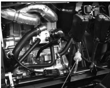
Fuel Tank Vent Filter
