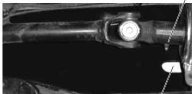
Fitting Access (as viewed from top with center floor panel removed)
