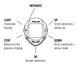
To adjust the data, use UP, DOWN and accept with OK. The values scroll faster if you press and hold UP or DOWN.
