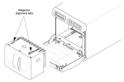
Figure 14. Inserting the Magazine
