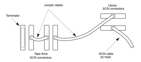
Figure 16. SCSI Bus Connections
