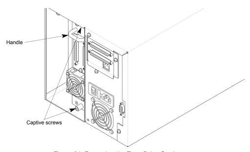
Figure 31. Removing the Tape Drive Carrier
