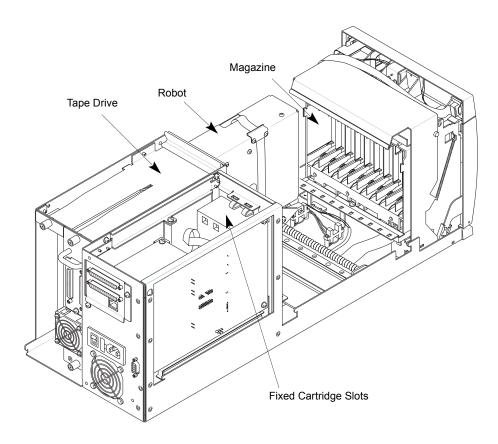
Figure 5. V15 Internal Components
