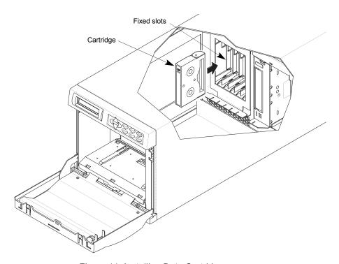
Figure 11. Installing Data Cartridges
