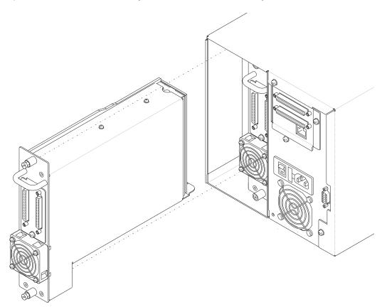
Figure 32. Installing a Tape Drive
