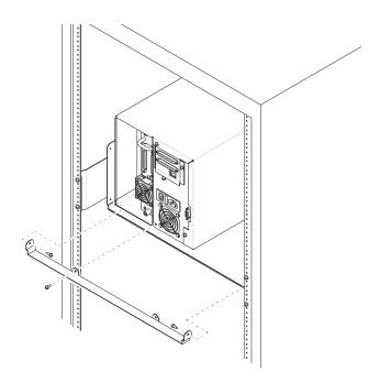
Figure 33. Removing Rack Mount Bracket
