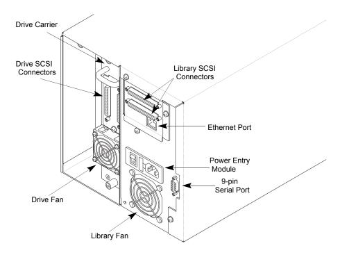
Figure 4. V15 Back Panel Components
