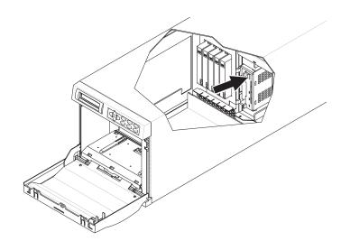
Figure 28. Tape Drive Eject Button
