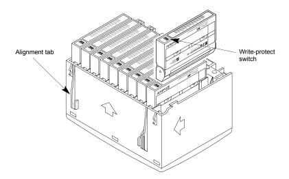
Figure 13. Installing Cartridges in the Magazine
