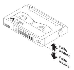
Figure 10. Data Cartridge Write Protect Switch
