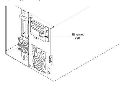
Figure 20. Ethernet Connector
