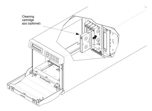
Figure 12. Installing a Cleaning Cartridge
