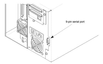
Figure 29. Serial Port Connector
