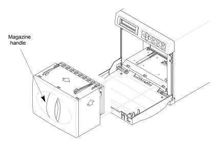
Figure 23. Removing the Magazine
