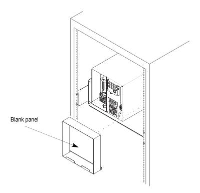
Figure 34. Removing Rack Mount Blank Panel
