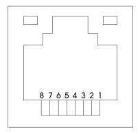
Figure 36. Ethernet Port Pin Locations
