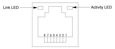
Figure 21. Ethernet LEDs
