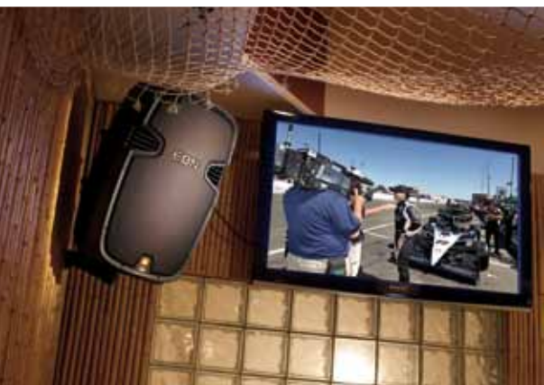
Top: The JBL EON portable speaker has a built-in amplifier, allowing easy placement throughout the restaurant for singers and bands.
