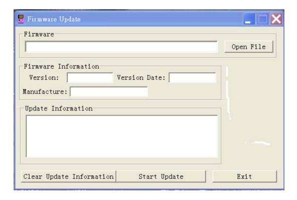
5. Connect the player to your PC using a USB cable (press and hold the Left key before the On-line operation), click [Burnt Firmware] until the Auto Upgrading is achieved.
