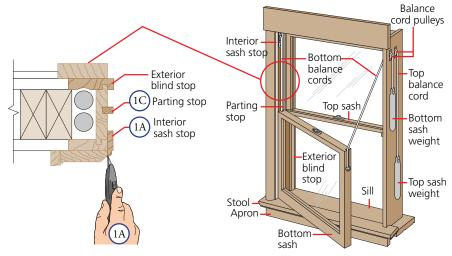
A. Score paint or varnish along interior sash stops with a sharp utility knife. Remove the interior sash stops at jambs (sides) and head (top) using a putty knife and pry bar.
