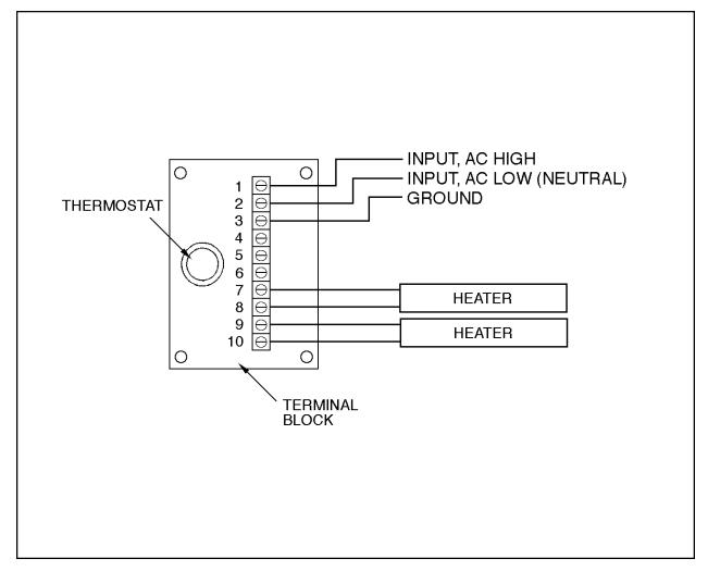
Figure 2. HKHS3000 and HKHS3024 Wiring Diagram
