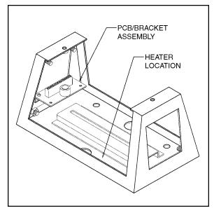
Figure 1. Heater Kit Installation
