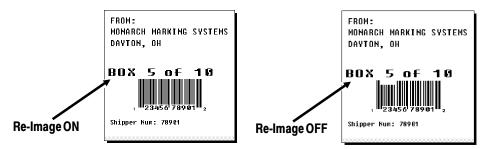
In the above example, Option 61 was applied to the bar code field to keep the incrementing field (Box #) from blocking out the bar code field.
