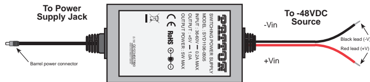
Figure 9. Connect DC power to the 48V-PSM3 DC power supply
