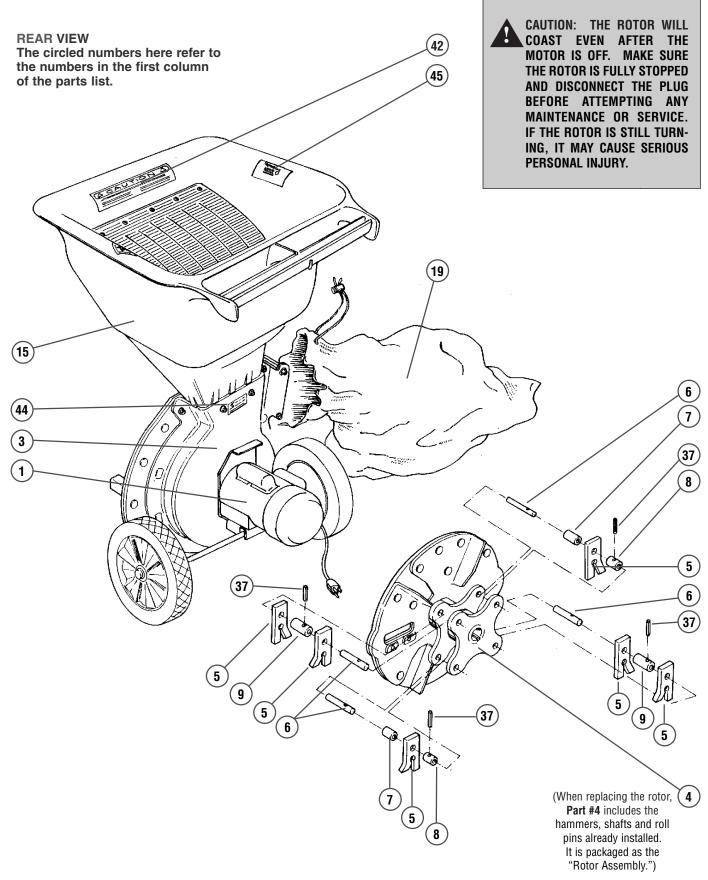
CAUTION: THE ROTOR WILL COAST EVEN AFTER THE MOTOR IS OFF. MAKE SURE THE ROTOR STOPS TURNING, THEN DISCONNECT THE PLUG FROM THE MOTOR BEFORE ATTEMPTING ANY MAINTENANCE OR CLEAN-OUT PROCEDURE. IF THE ROTOR IS STILL TURNING, IT MAY CAUSE SERIOUS PERSONAL INJURY.
