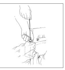
Now check all the fasteners. They may have loosened during shipping. Tighten anything that's loose. It's a good idea to check the fasteners for tightness before every use.
