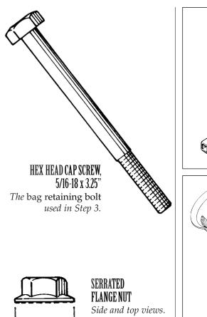
Side and top views. The serrations on the bottom bite into the steel for better staying power.
