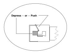
Fig. 11: SIM Socket Clip - Top View
