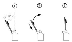
Fig. 10: I/O Board Insertion
