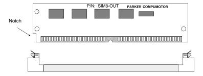
Fig. 9: I/O Board and Socket
