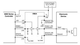
Note: Make sure the jumper between OUT-P and +5V on the 6000 Series unit is removed to avoid damage to the VM24
