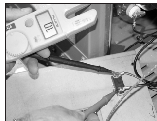
Testing the door push-button safety switch.
