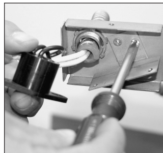
Loosen switch mounting plate.
