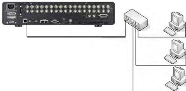
Figure 1-4 Network Connection through Patch Cable
