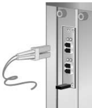
FIGURE 2-3 Connecting the Optical Cables
