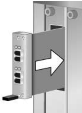
FIGURE 2-2 Inserting the HBA Into the AMC Connector
