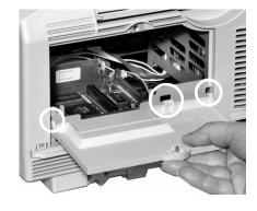
b. Swing the panel up and tighten the screw to secure it in place.
