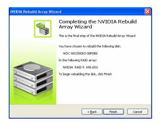
7. Click Finish to begin the rebuild of the selected disk in the array. (Remember that rebuilding a disk can take up to a full day.)
