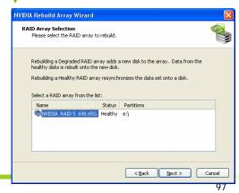
healthy disk is rebuilt onto a new disk.
