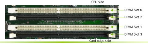
Use the following procedure to install memory DIMMs into the slots on the motherboard. Note that there is only one gap near the center of the DIMM slot. This slot matches the slot on the memory DIMM to ensure the component is installed properly.
