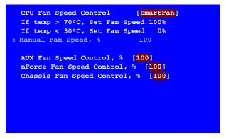
Use this menu to control the speed of the various fans on the motherboard. Set CPU fan speed to [SmartFan] when you want the speed of the fans automatically controlled based on temperature. To set the fan speed to a constant rate, select [Manual] and then enter the speed from 0% to 100%.
