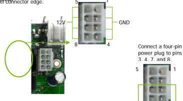
It is *strongly* recommended that you use an 8-pin ATX 12V power supply; however, if you have a four-pin power supply, plug the connector to pins 3, 4, 7, and 8 as shown.
