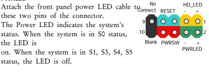
**Note:** The power LED cable in some chassis is a three pin connector with the pins installed in positions 1 and 3. If your chassis has a three pin connector, you will need to remove pin 3 and put it into position 2 or you can use a pair of scissors to cut out position 2. Most chassis come with a two pin connector.
