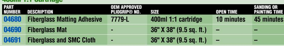
USE APPLICATOR GUN #41398-MANUAL OR #41396-PNEUMATIC. USE 24 ELEMENT MIXING NOZZLE #04628.
