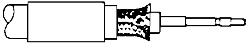
Figure 13: Flared cable braid
