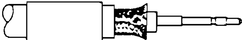
Figure 8: Flared cable braid
