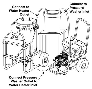
7. Run the pressure washer in cold mode for 1 to 3 hours recirculating the cleaning solution.
