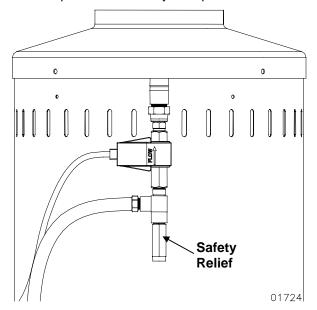
WARNING: If the safety relief valve ever discharges water, turn the unit off and do not use the machine. See a dealer or call Customer Service at 1-800-270-0810.
