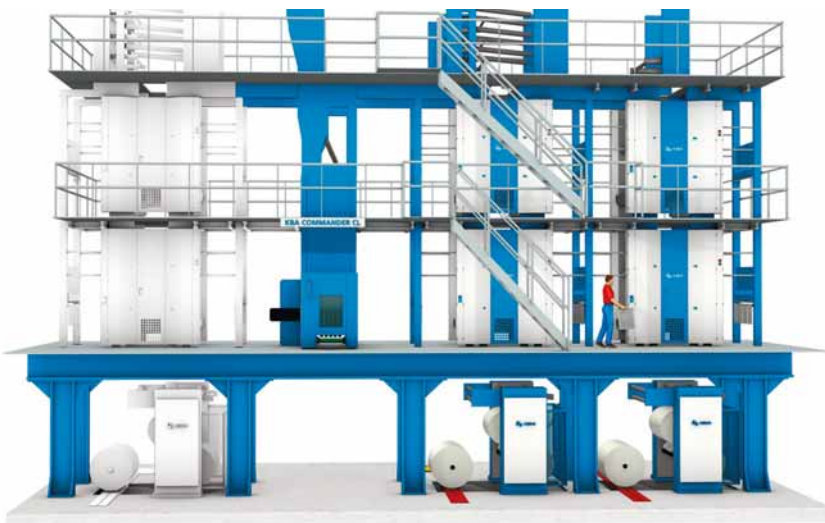
3-D schematic of the 4/2 KBA Commander CL for the Gelnhäuser Neue Zeitung
