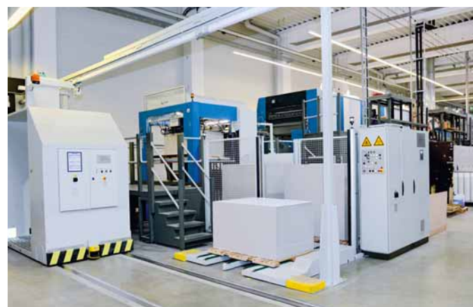
Automatic pile logistics at the Rapida 145 feeder
