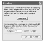
$2^{\text{Straighten the image}}$  Straighten the image using the  $^{\text{Draw Level}}$  button or by entering the desired rotation in the  $^{\text{Rotation}}$  text box.
