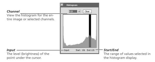
To select an area of the histogram, drag the mouse over the histogram display. The pixels with values in the selected range will blink in the image window. Click **Clear** to cancel the current selection.
