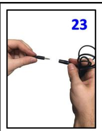
**Step 23:** Connect the Swivel Cable coming off of the Swivel Mechanism to the 6' Adapter Cable.
