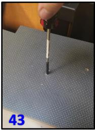
**Step 43:** Using a Phillips head screw driver (not provided) screw each Tapered Pin into the holes drilled in step 16.
