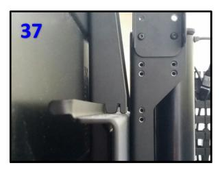
**Step 38: Insert both** *Screen Locks* **into both** *Vertical Mounting Bars.* Using (2) *Screen Locks*, place one *Screen Lock* on the bottom set of hooks for each *Vertical Mount Bar*. Using a Philips Head Screwdriver (not provided), tighten the *Screen Locks* against the bottom of the *Screen Back Plate*. This will ensure the TV does not slide left to right and eliminate the TV from being lifted off of the mount.
