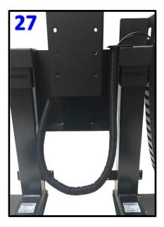
**Step 28:** Push the Snakeskin Wrap up through the Right Cable Management Bracket, slide Right Cable Management Bracket to the right the pin the cables against the Center Riser Bracket, and tighten the (2) 6 x 20 FHMS Screws.
