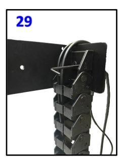
**Step 29:** Attach the right half of the Cable Management Track to the Rear Support Bracket using (2) 5 x 12 mm FHMS Screws.
