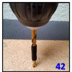
**Step 42:** Remove Cabinet Lid and drill two holes in the marked positions using a 7/32'' drill bit,  $\frac{1}{2}''$  deep, in the underside of the Cabinet Lid.
